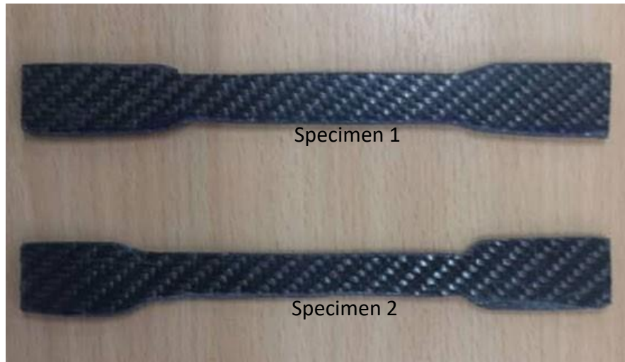
Figure 1. The fabricated test specimen for Tensile Test
