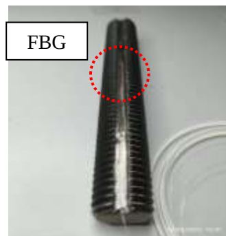
Figure 3. Location of FBG on bolt.
