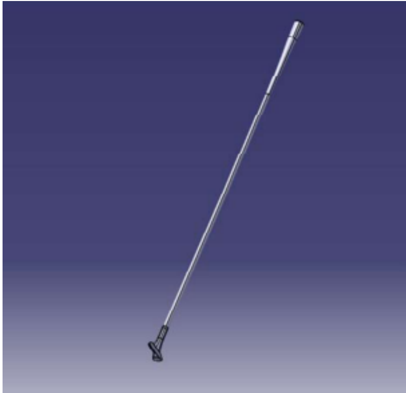
Figure 2: CAD model of the golf club-the completed CAD model, exported in Parasolid format, forms the geometric basis for the subsequent FE and EMA investigations.
