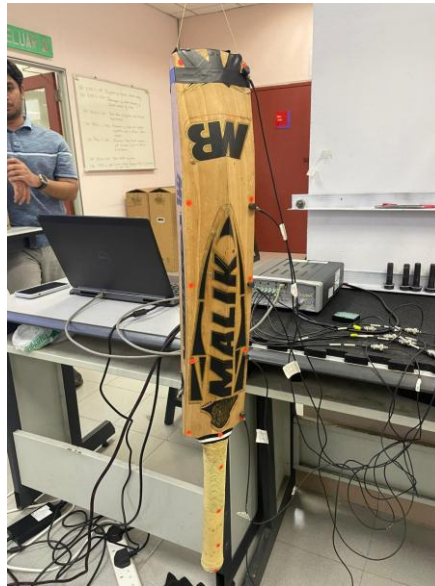
Figure 8. EMA setup of the physical cricket bat
