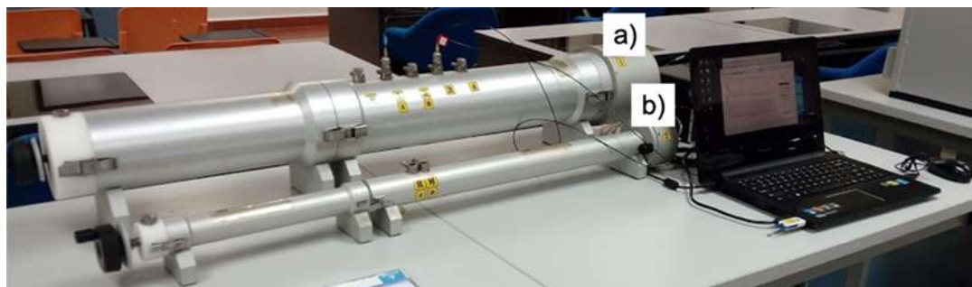
Figure 2. Impedance tube model Kundt tube type SCS9020B. a) A 100 mm diameter test tube; b) A 28 mm diameter test tube.
