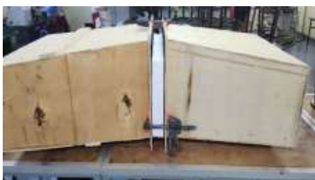
Figure 3. Chamber being clip together with the sample in between
